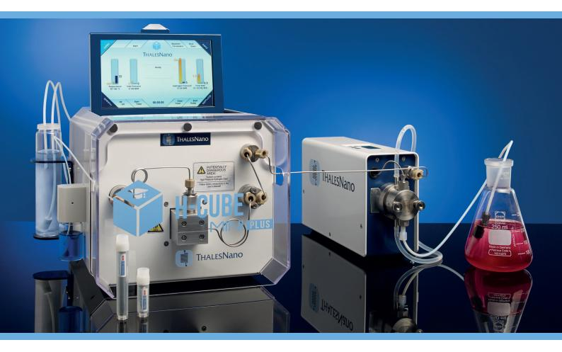
Safe: No H<sub>2</sub> cylinders and catalyst filtration Powerful: 100 °C and 100 bar capable Fast: results in 4 minutes Simple with built-in video tutorials
